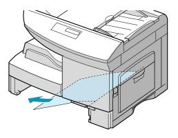
If you remove the jammed paper here, open the side cover then close it to clear "PAPER JAM" message on the display.
